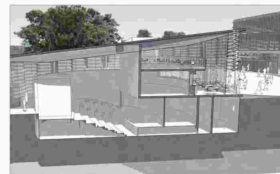
Section through the 'Community Hub' showing the auditorium, restaurant and civic square (underground parking is not shown)
